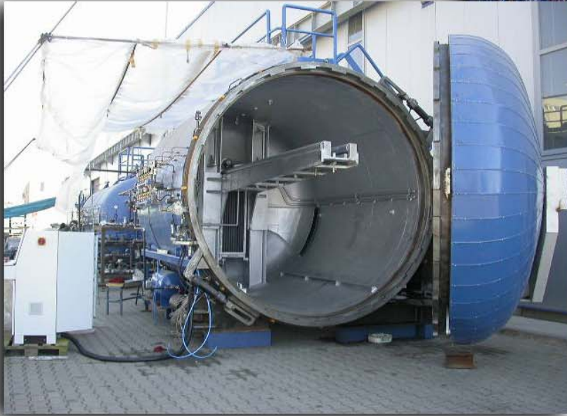
Diameter: ø3100 mm Length: 3955 mm
